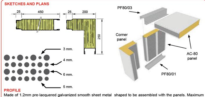
length of 3000mm. Special thickness of 2.5mm for barriers and special installations.
